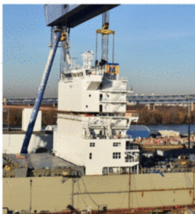
Installation of the deck house with navigation bridge on the first Aloha Class ship.
