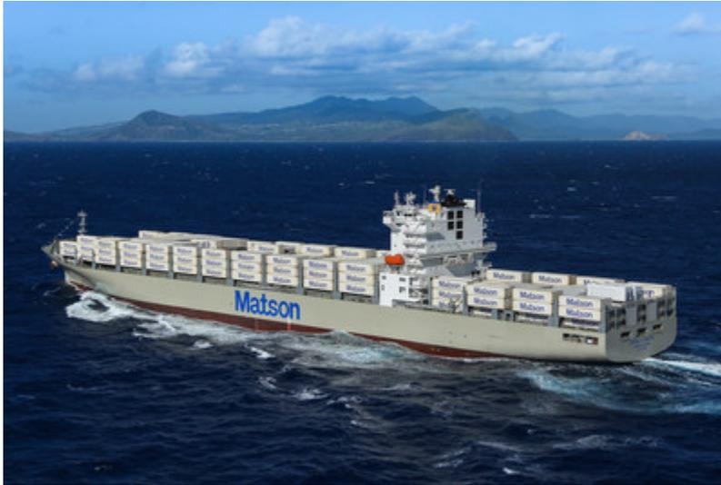
Named in honor of Hawaii's late senior U.S. Senator, the *Daniel K. Inouye* is the largest containership ever built in the United States. Weighing in at over 51,400 metric tons, the 850-foot long, 3,600 TEU\* vessel is Matson's largest ship and also its fastest, with a top speed in excess of 23 knots.
