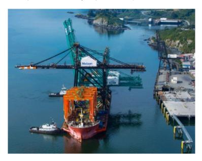
Standing more than 340 feet tall at its peak with a boom spanning 164 feet, Matson's new crane is the largest in Alaska, capable of lifting loads up to 60 feet long and weighing up to 145,000 pounds.
